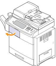
2 Pull the stacker lever **1a** down. If necessary, pull the stacker lever **1b** down as well.
